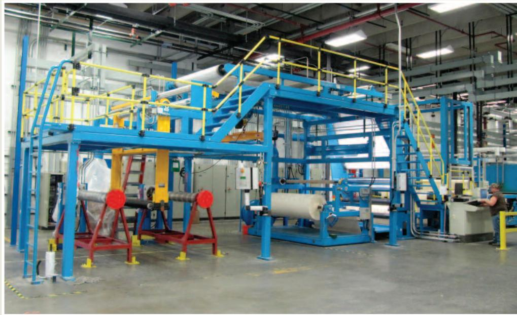
Winder section of the new artificial leather manufacturing facility. This production line was completed in September of 2011. It produces films to be used in all forms of transportation, furniture, wall coverings, and similar products.
